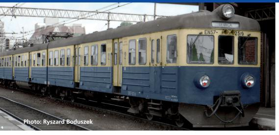
Between 1961 and 1993, 1,412 sets of the electric railcar of the class EN57 were built by Pafawag, the state-owned Polish wagon factory in Wroclaw, for the Polish state railways.
